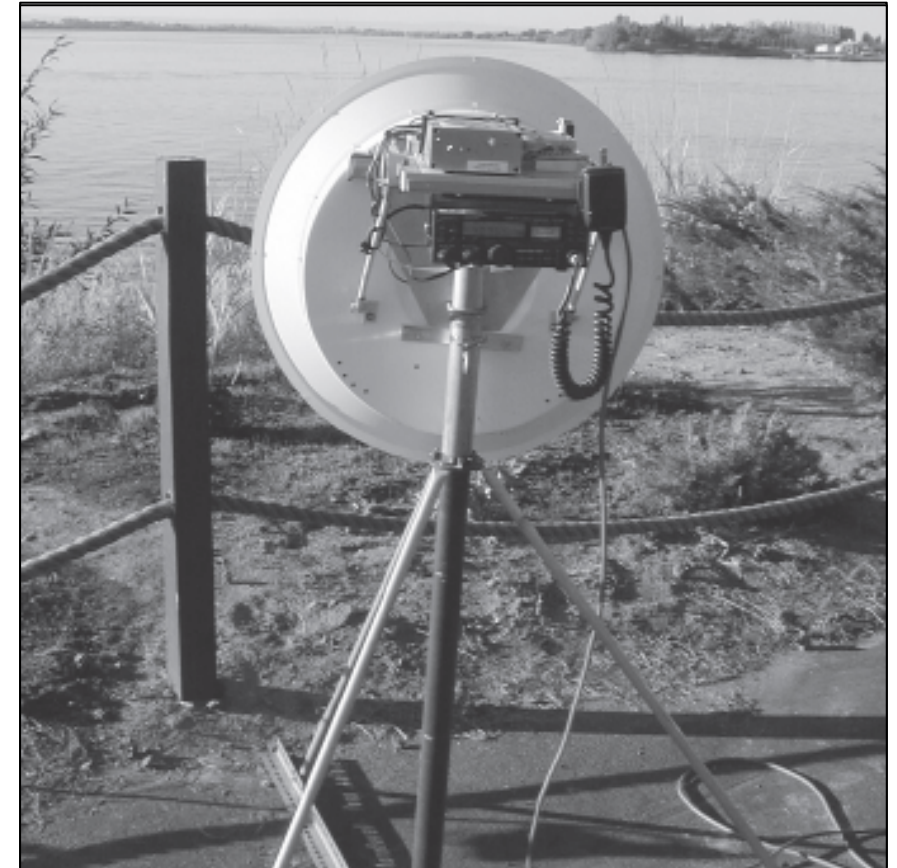
Figure 4.14 — N7CFO's dish antenna operates on 10 GHz and is portable enough to be taken on contest outings.
