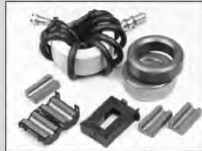
Figure 9.4 — Ferrite is a ceramic magnetic material used to make choke filters for RFI suppression. It is available in many different forms: rings (toroids), rods, and beads. Cables can be passed through or wound on these cores to prevent RF signals from flowing along their outside surfaces.
